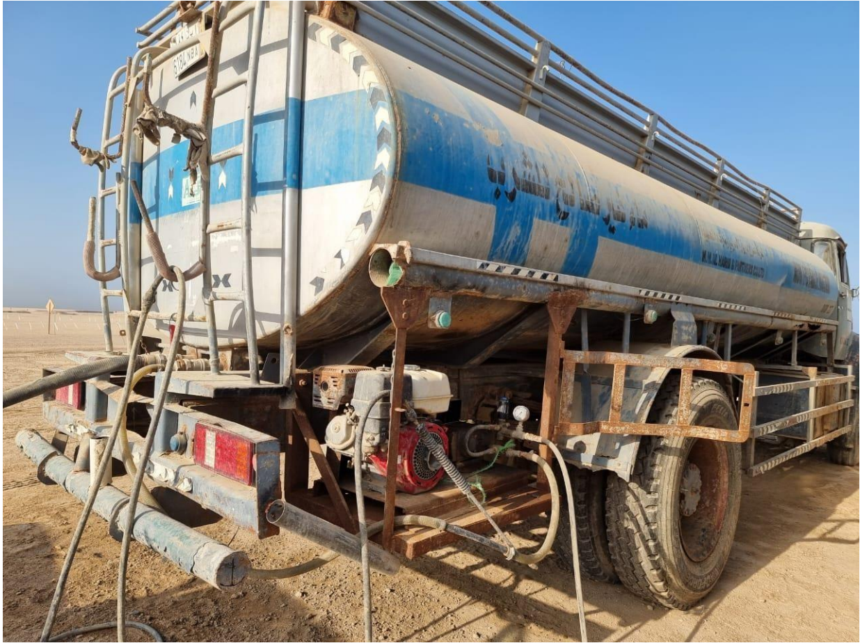
Figure 6. Fire hose fittings attached to water truck.
